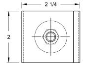
SEISMIC VERTICAL LIMIT-STOP, NUT AND WASHER, TIGHTEN TOGETHER (SEE NOTE 3)
